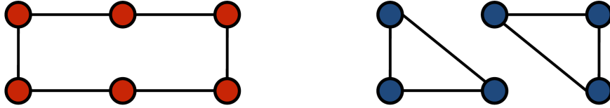
Figure 7.3: Example of two graphs that cannot be distinguished by the basic WL algorithm.
