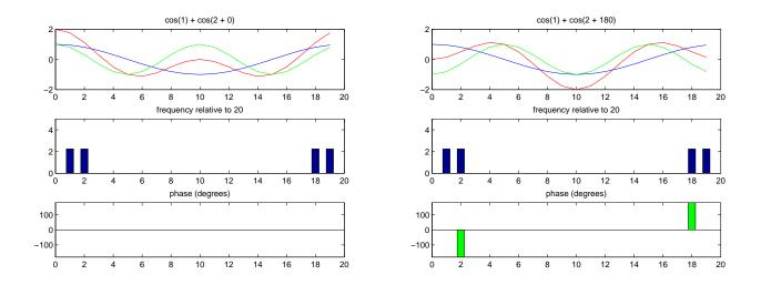
23. **Two-dimensional discrete Fourier transform** The two-dimensional waves of Note 22 in Book 8c (part II) can be used in a two-dimensional Fourier transform
