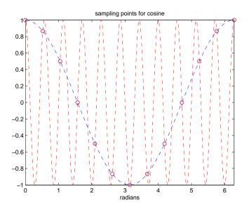
Explore this for different frequencies, including those greater than 12. Why must the sampling rate be at least twice the highest frequency one needs to detect? c) Modify your program to interpret negative frequencies by their absolute values but with the phase altered by  $\pi$ . Explore the sampling now.
