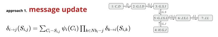
calculate the beliefs **in the end**  $\beta_i(C_i) = \psi_i(C_i) \prod_{k \in Nb_i} \delta_{k \to i}(S_{i,k})$
