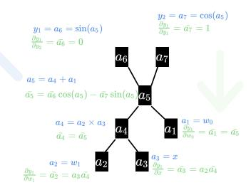
forward mode is more natural, easier to implement and requires less memory a single forward pass calculates  $\frac{\partial y_1}{\partial w}, \dots, \frac{\partial y_c}{\partial w}$
