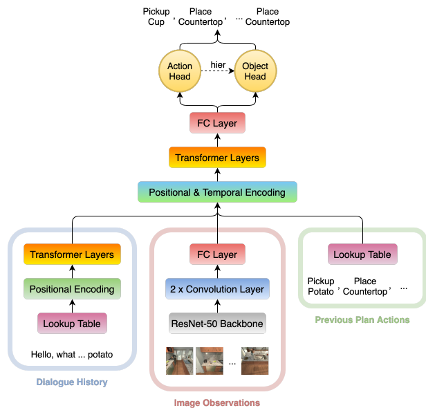
Figure 2: This is a depiction of the architecture for the E.T.-based models. The basic E.T. model does not have a connection between the action and object heads, but E.T. Hierarchical does. There are three main input processing components (dialogue history, image observation and previous plan actions). These are then input into the positional and temporal encodings and transformer layers to come up with the next feasible set of high level plan actions.
