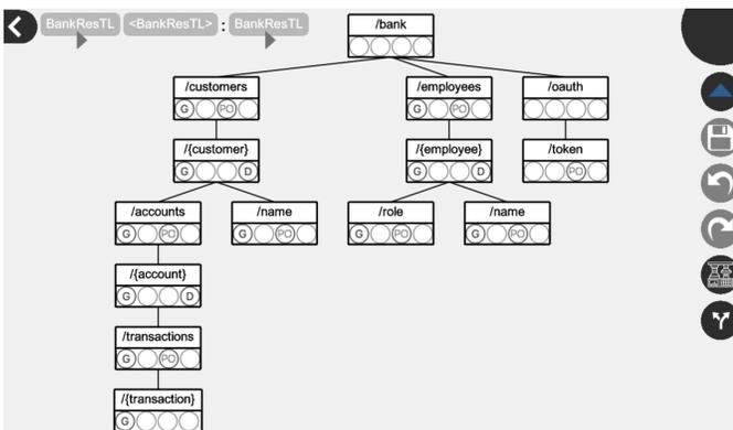
Fig. 4. ResTL Model Defining REST Resources and Methods for the Bank
