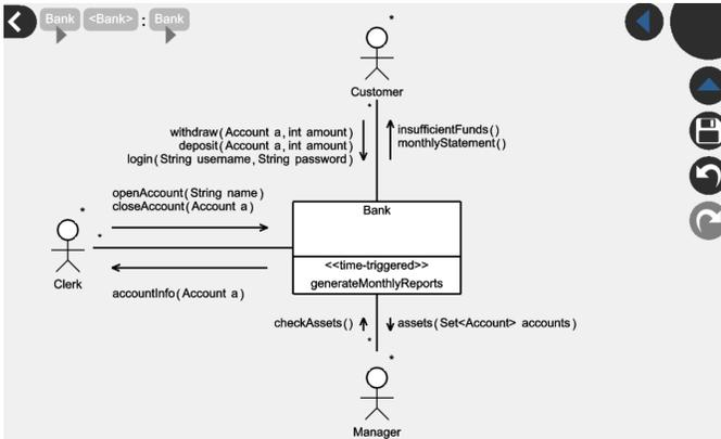
Fig. 3. Environment Model of the Bank
