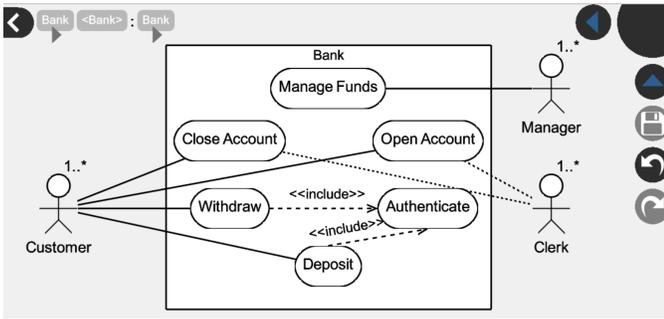
Fig. 2. Use Case Model of the Bank
