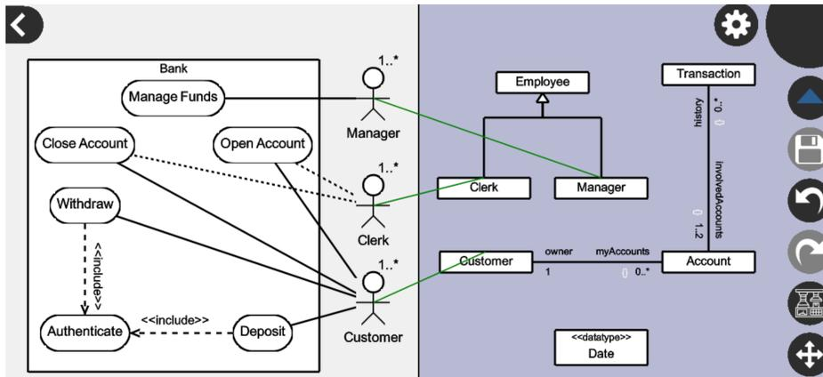
Fig. 6. Use Case Model and Domain Model Visualized Side-By-Side Using the Generic Split View
