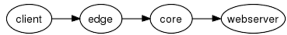
Figure 6: Test topology designed to stress the HRT load-balancing content-based routing protocol. HRT entries were set to time out quickly after being updated so that the Edge router would continuously send HRT requests for the content to web server mapping.
