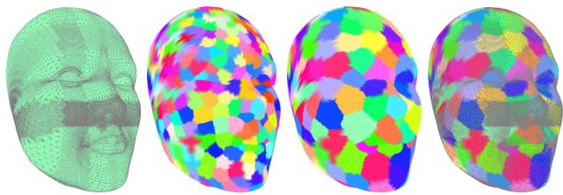
**Figure 2:** An example mesh with two different resolution partitions into uniform regions. Our greedy algorithm is unaffected by varying density in the mesh. Region centers define the locations for overlapping Gaussian weighted averages that make up our constraints.
