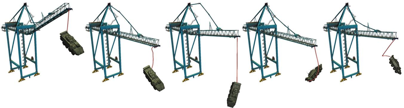
**Figure 1:** A heavy vehicle attached to a nearly inextensible cable is dropped from the end of a crane. The simulation involves very large mass ratios, a heterogeneous collection of joints, and remains stable at a time step of  $1/60$  s. Cable dynamics are well preserved by our adaptive damping method.
