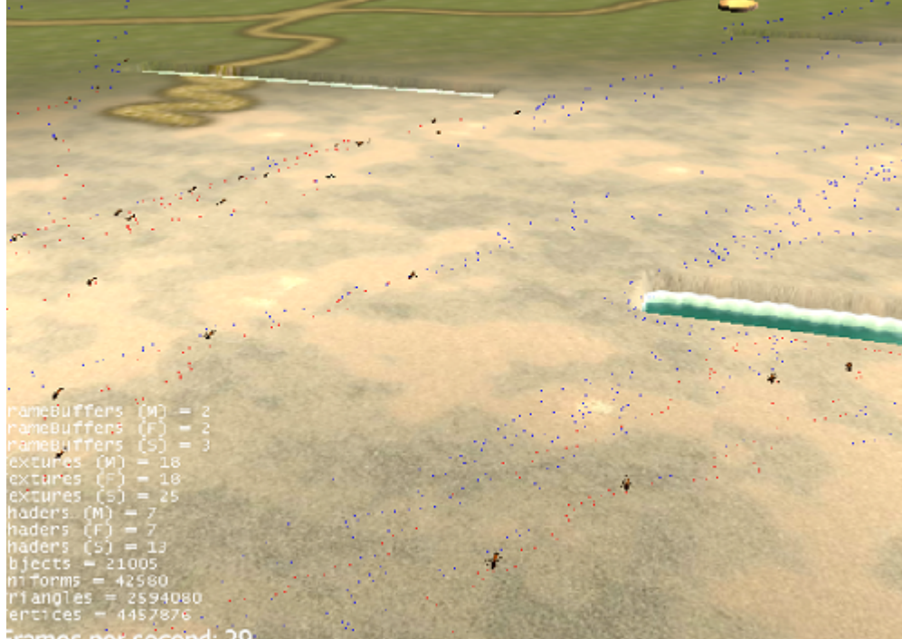
Figure 5-5: Initial Reinforcement Phase: The pheromone deposits of the recruits are shown by red dots and the pheromone deposits of the recruiters are shown by blue dots. This snapshot shows recruits following the pheromone trails established by the recruiters. During this phase, the recruits will have just started and that's been reflected by the fewer number of red dots. The blue dots present all over represent the different routes taken by the recruiters. Here, it can be seen that initially the recruits don't show any preference any of the recruiters' paths as it only happens gradually.
