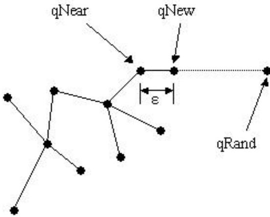
Figure 1: RRT Expansion process.  $q_{rand}$  is a randomly chosen point,  $q_{near}$  is its nearest neighbor in the tree. The local planner is only allowed to progress a distance  $\epsilon$ , after which a new point is added and the process repeats.
