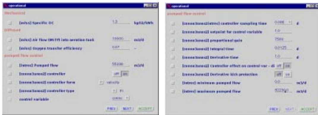
Figure 6.11: Dialogue boxes showing the implementation of the nitrate controller.
