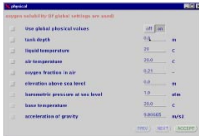
Figure 6.5: The GENERAL DATA menu 'physical' dialogue box showing the required DO parameter values to achieve a DO saturation concentration of 8 g m^{-3} .
