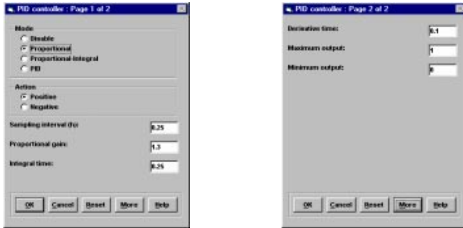
Figure 8.6: Nitrate PI controller settings.
