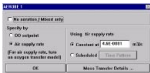
Figure 4.7: Bioreactor dialogue box (BioWin version 4.4b) for the AEROBE 1 reactor - see Figure 4.2 – showing the required air supply rate to attain a K_La of 10 \text{ hr}^{-1} in that bioreactor.
