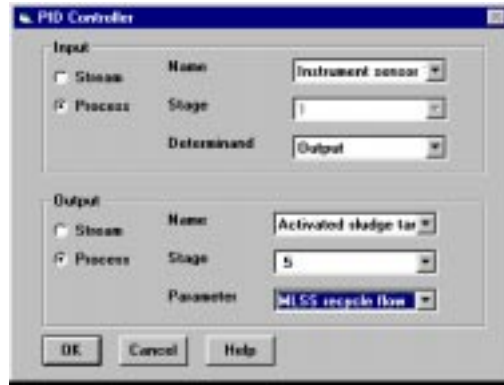
Figure 8.5: Nitrate PI controller signal set-up.
