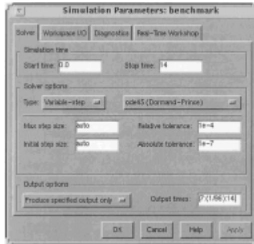
Figure 7.2: Explicit results output times have been specified in the simulation parameter window. Results are saved from day 7 to day 14 with a time interval of 1/96 day = 15 minutes.
