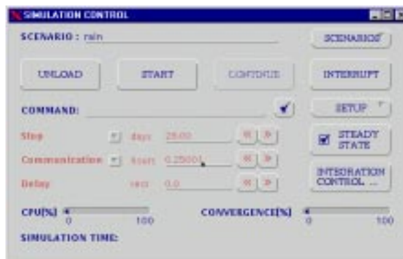
Figure 6.8: 'Simulation control' dialogue box showing the use of the steady state solver option, the use of the necessary 0.25001 hours 'communication interval' and the 28-day simulation time.
