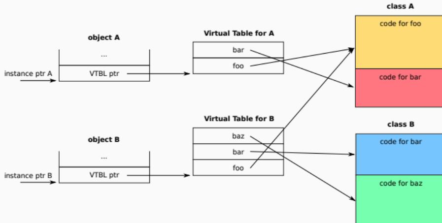
Assuming variable p declared with type A, code for p.bar():
