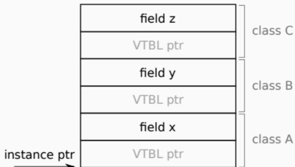
There is one virtual table for each super class in the object and the virtual table is chosen based on the static type of the instance **ptr**.
