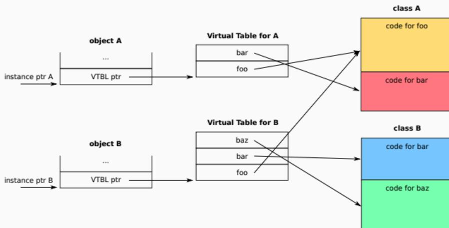
Inherited methods from the superclass are at the same fixed position in the virtual table.
