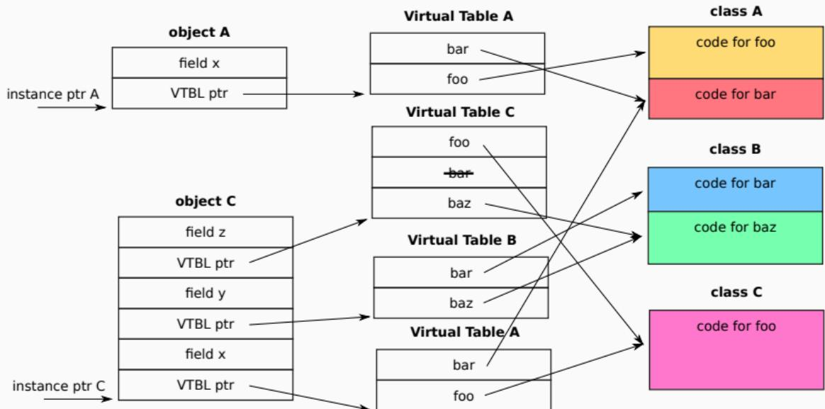
Key property: instance methods of given class are always in the same location in the corresponding virtual table.
