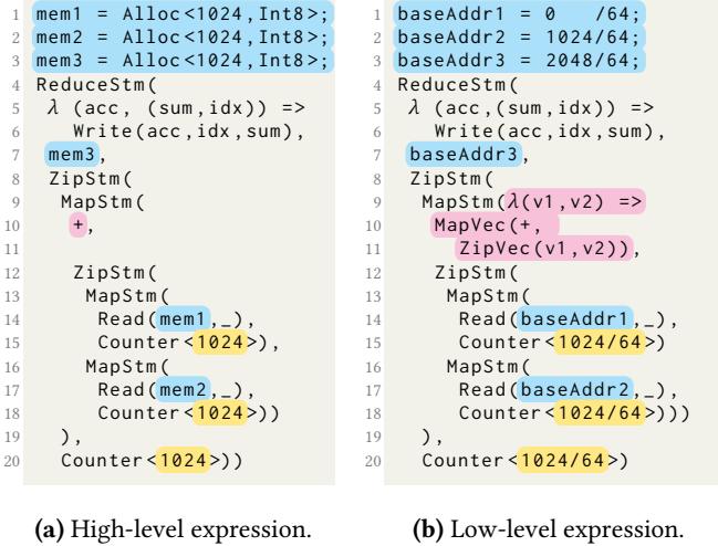
Figure 4. SHIR expressions for adding two arrays in memory. x = a ; e is syntactic sugar for a Let construct: Let x = a in e . Type parameters are passed inside \langle \rangle while function arguments are passed inside () .
