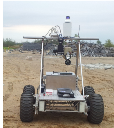
Figure 1. IVIGMS LIDAR (white box on top of the rover mast) on the Juno rover at CSA Mars Yard in 2012.
