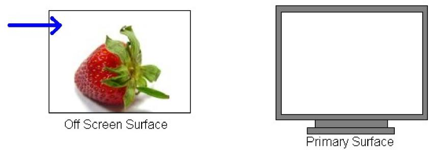
2. Copy the content of the off screen surface on the primary surface (screen).
