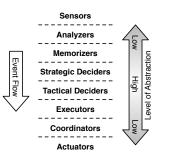
Fig. 1. AI Model Architecture
