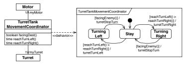
Fig. 13. Coordinating and Controlling the Turret
