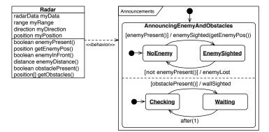
Fig. 5. Generating Events based on Simple Computations
