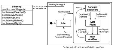
Fig. 12. Steering the Tank
