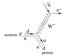
Neutrons and protons consist of up-quarks and down-quarks, three each. A neutron becomes a proton by one of its d-quarks becoming a u-quark by emitting a  $W^-$  boson which then decays into an electron and an antineutrino. Note that, unlike the photon at the end of the previous Note, which is neutral, the  $W^-$  boson carries a (negative) charge, in order that electric charge be conserved at each vertex.
