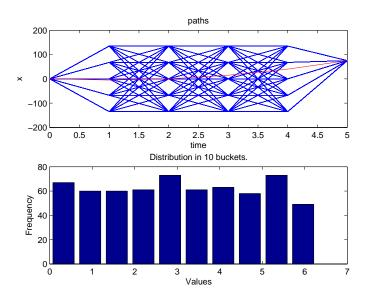
You can see that the particle is not forbidden any location in space (apart from the finiteness of the simulation). It can move from  $x_a$  towards  $x_b$  or away from it, and similarly for each step until the last, when it must arrive at  $x_b$ .
