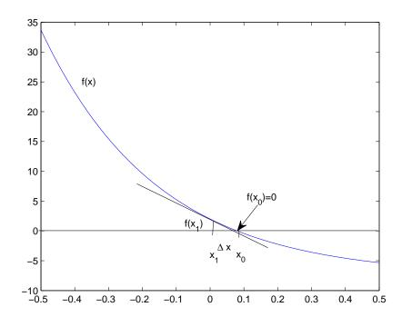
The figure shows why we must have the minus: the slope of the curve in the figure (it is just the above expression we are trying to solve for  $\beta$ ) is negative, so  $\Delta x \approx x_1 - x_0$  is negative if our first guess is  $x_1$  as shown. So to advance to where the black line crosses the x-axis in the figure (about 0.08) we must subtract  $\Delta x$  from  $x_1$
