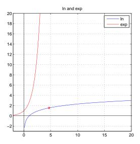
This plot also shows the closely related function "exp()", the "exponential". You can see where to put a mirror in this plot which would reflect the blue curve into the red curve and vice-versa.
