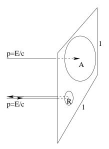
It is made of very thin, strong material, such as aluminized mylar (areal density  $\sigma = 7$  grams per square meter) or, ten thousand times better, graphene (a carbon monolayer with areal density  $\sigma = 0.7$  milligrams / m<sup>2</sup>). It will either absorb, reflect or transmit a photon, in the respective proportions A, R or T = 1 - A - R.
