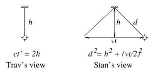
Stan sees the light travel upwards then downwards on diagonals, taking time t where  $c^2t^2=2^2d^2=2^2h^2+v^2t^2$ . Show that  $t=t'/\sqrt{1-(v/c)^2}$ .
