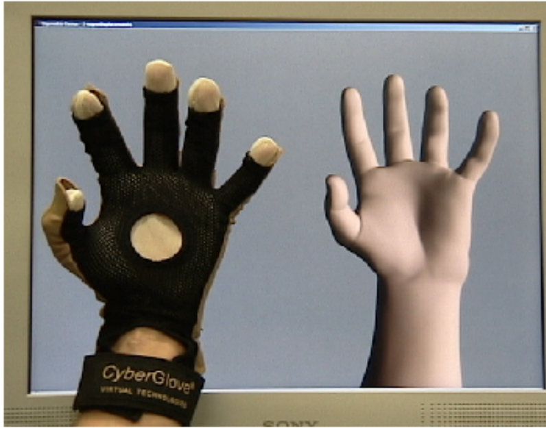
Figure 7.10: An EigenSkin hand example being animated using a CyberGlove. The hand model shown here consists of 55,904 triangles and is drawn using display lists with a vertex program.
