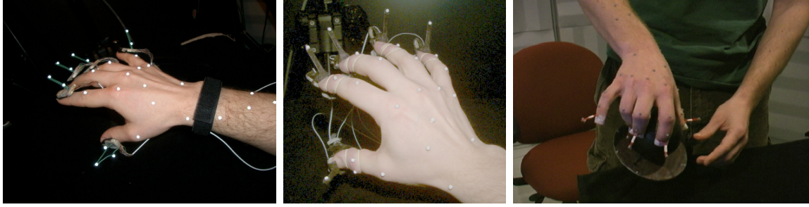
Figure 3.1: Markers on the distal phalanx are placed on stilts rather than the fingertip, shown on fingernail sensors (left), force sensitive resistors (middle), and attached to the fingertip (right). This improves marker visibility during grasping.
