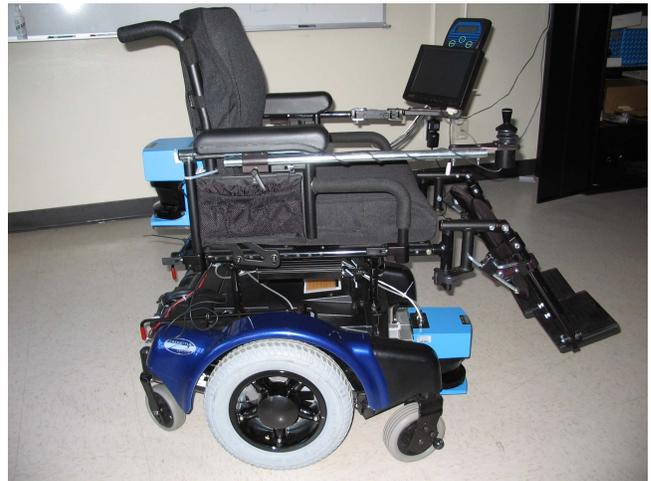
Fig. 6. The SmartWheeler Robotic Wheelchair
