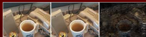
Two frames and the optical flow field that maps pixels from one frame to another
