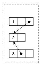
Heap variables may be referred to by other objects in the heap, or from the stack.
