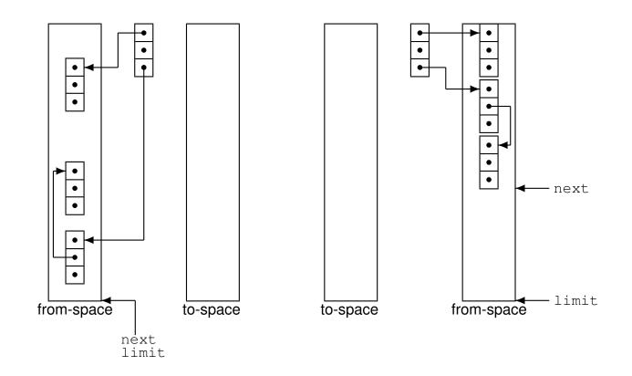
The stop-and-copy algorithm internals are much more complicated. Intuitively, it *forwards* each record on the heap in a breadth-first manner (starting from the stack).
