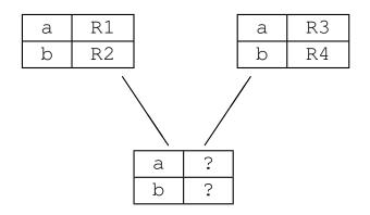
To correctly merge the paths, registers must be spilled after basic blocks
