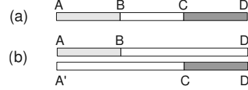
Figure 5: Elements with disconnected material (a) are split in distinct, initially superimposed elements (b).
