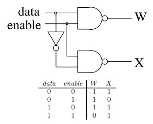
Now the flipflop just remembers the value data had when enable was set to 1. What it remembers is always available on Y (the output from the flipflop on the first page, whose input is W and X). Here it is in MATLAB.
